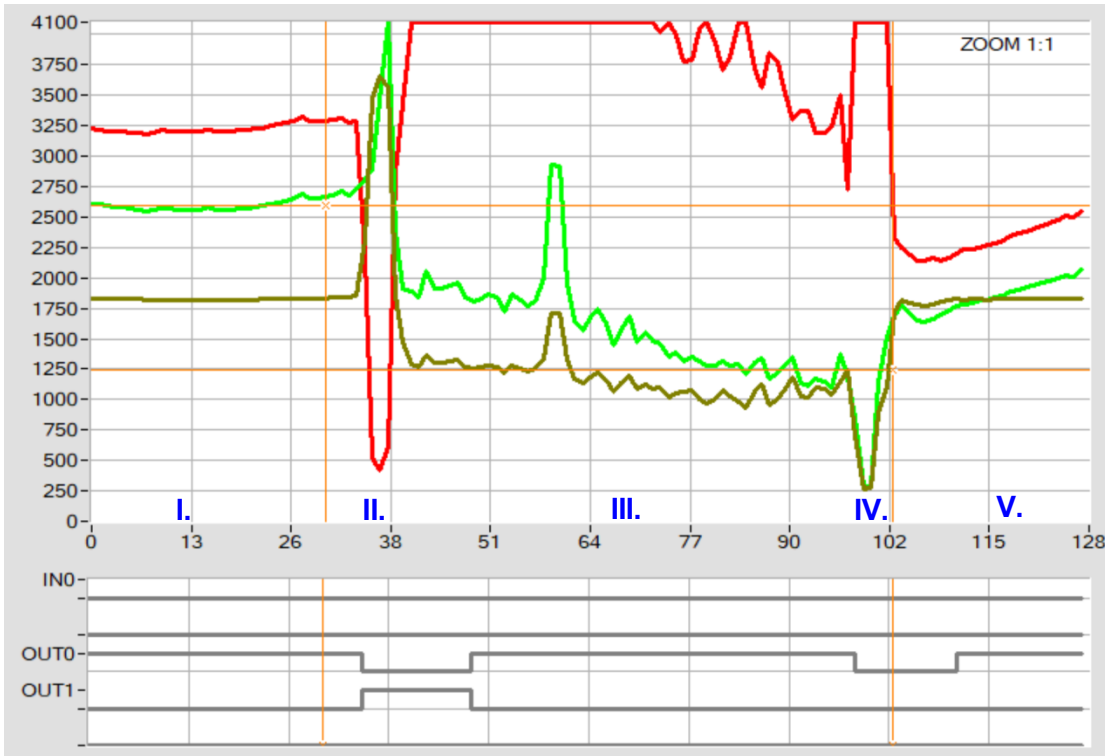
Image-6: SIG, CH0, and CH1 while moving another test sample with a more shiny surface underneath the sensor. OUT0 and OUT1 are extended to 100ms (software adjustable HOLD time), once SIG is cutting the lower threshold (rising edge) or the upper threshold (falling edge).
