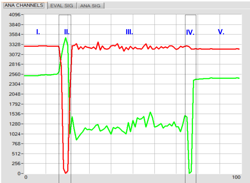
Image-4: ANA CHANNEL (CH0, CH1) conditions while moving the test sample underneath the sensor
